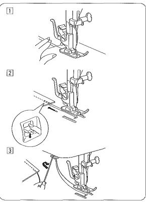
1 Raise the presser foot and position the fabric with its edge lining up with a seam guide line on the needle plate.
