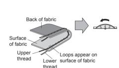
**Solution:** Reduce the tension by turning the upper tension control dial to a lower number
