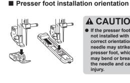
**A** CAUTION If the presser foot is not installed with the correct orientation, the needle may strike the presser foot, which may bend or break the needle and cause
